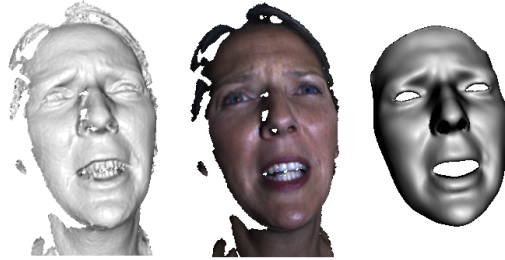
Fig. 2. From left to right, the image shows the 3D reconstruction of a person's face, the corresponding texture mapped on it, and the personalized face templated deformed to fit the specific frame.
