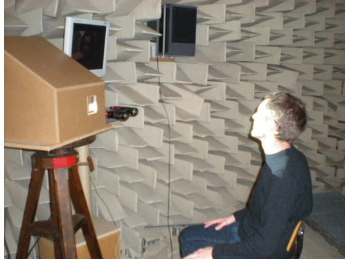
Fig. 1. Recording setup: one speaker sits in front of the 3D scanner in the anechoic room while watching one of the eliciting videos clips.
