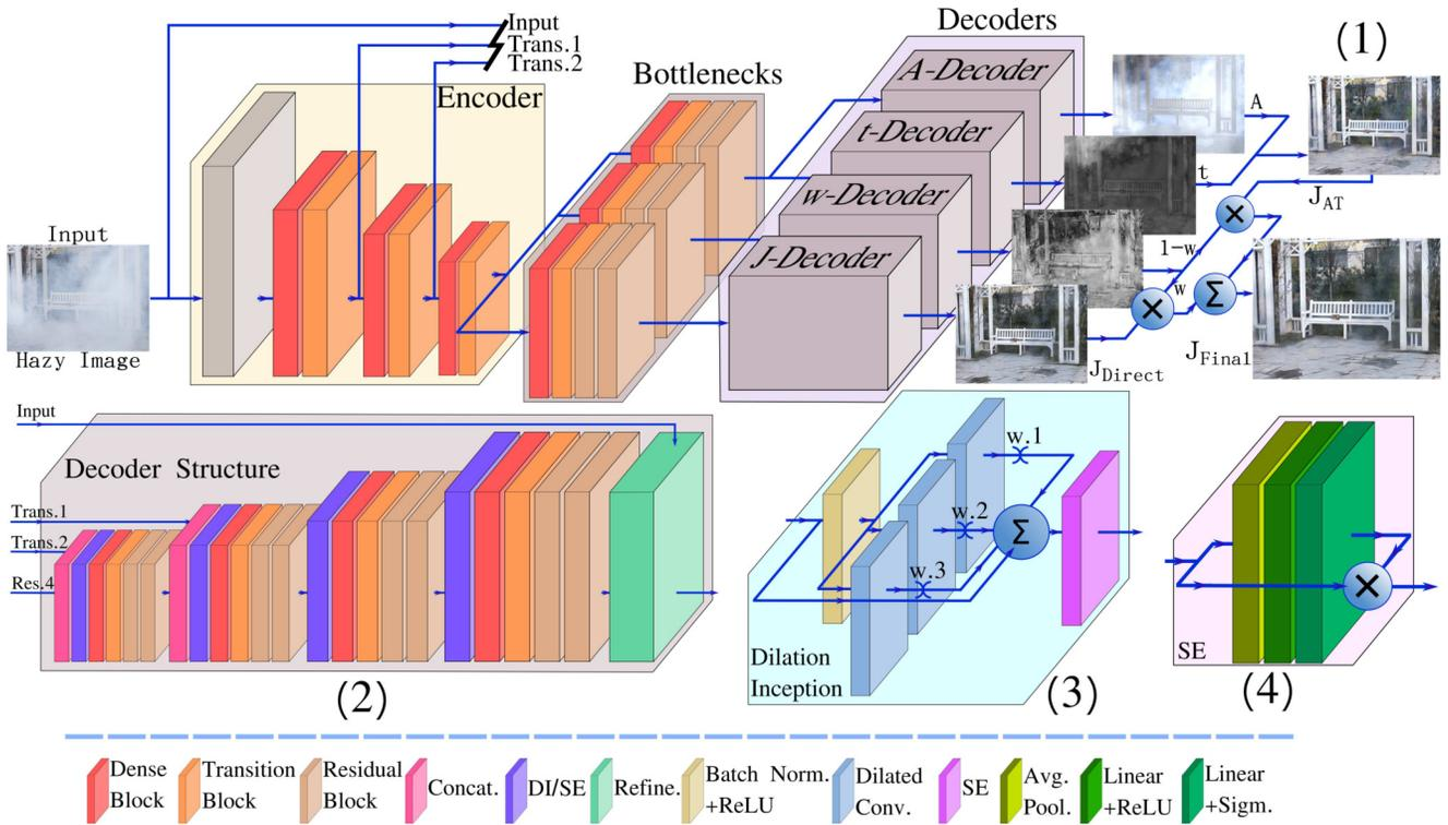
Figure 10: Overview of the method introduced by iPAL-NonLocal. All decoders are identical except for  $J$ -Decoder which has extra layers for non-local features utilization (Dilation Inception-DI).  $A$ -,  $t$ - and  $w$ -decoders only use SE layers.
