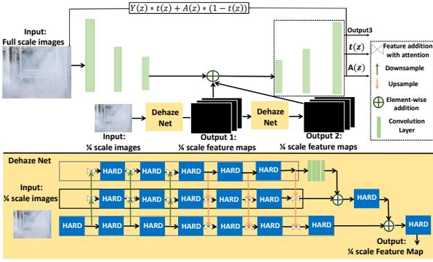
Figure 5: Overview of the framework introduced by **de-haze.sneaker** team. It contains one encode-decoder framework for full scale images processing, while DehazeNet is proposed to handle  $\frac{1}{4}$  scale images to provide haze-free information to framework. In the bottom are shows the details for DehazeNet.  $\frac{1}{4}$  scale images are feed into the DehazeNet.
