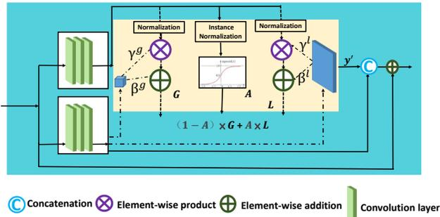
Figure 6: **Haze-Aware Representation Distillation (HARD) Module**. HARD is composed of two branches. The second branch is used to learn spatial information  $\gamma_g$ ,  $\beta_g$  and global atmospheric light information  $\gamma_l$ ,  $\beta_l$ , then feed them into the first branch to form intermediate results  $y'$ . After channel attention, the final result of HARD is produced.
