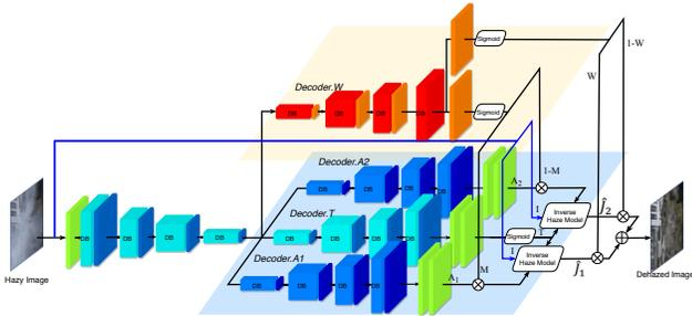
Figure 12: Overview of the method proposed by iPAL-EDN team. In EDN-AT model, ambient light maps  $A_1$ ,  $A_2$ , transmission map  $t$  are estimated by decoder.A1, decoder.A2 and decoder.T respectively.  $A_1$ ,  $A_2$  are multiplied by attention maps  $m$  and  $1 - m$ . Final output is a weighted combination of two sub-models' outputs.
