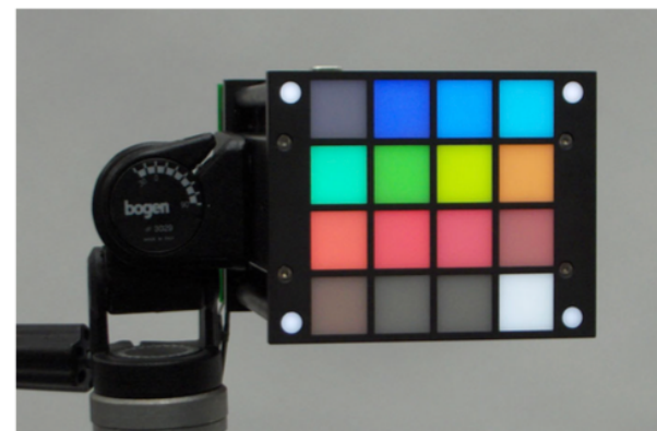
Figure 6. The first prototype of the emissive calibration chart.
